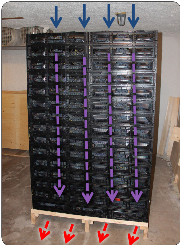
Figure 3. This column vertical airflow system uses RPCs with bottom vents. Cold air (blue arrows) is pulled vertically down from the top of the stack (purple then red arrows) through a specially designed pallet using a high-capacity fan located at the base (not shown). RPCs work well because they have fully vented bottoms, cross-stack on alternating layers, fit perfectly on a standard pallet and fit so tightly against each other that there are no spots where cold air can short-circuit. All four vertical sides of the stack must be covered with tarps (not shown) to compel cold air to travel vertically. (Photo courtesy of Dr. Bernard Goyette, Vineland Research and Innovation Centre, Vineland)
